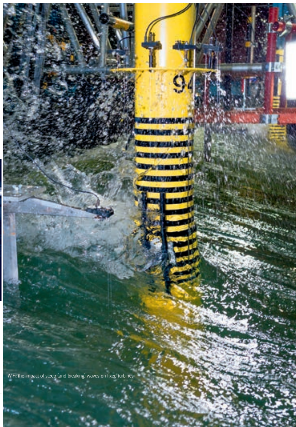
Short-crested wave impact on a fixed platform deck as measured during the ShorTCresT JIP
